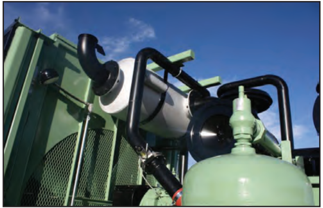
(Left) Each of the three engines are integrated into a single operator station that can be operated from the ground level. (Right) A view of the spark-arresting muffler on the QSX 15 Cummins engine and the overspeed/air shutoff valve.
