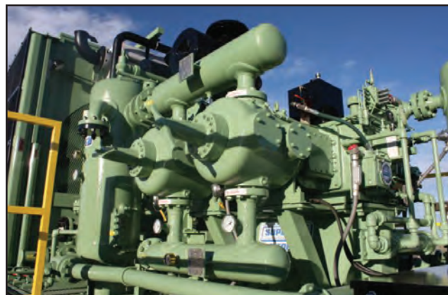
A view of the Superior C-Force three-stage, four-throw booster compressor frame and cylinders.
