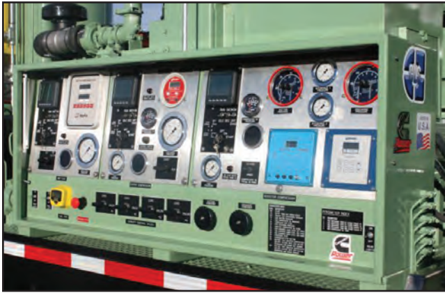
(Left) Each of the three engines are integrated into a single operator station that can be operated from the ground level. (Right) A view of the spark-arresting muffler on the QSX 15 Cummins engine and the overspeed/air shutoff valve.
